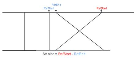
Figure 34. Estimation of inversion size on inversion/inversion\_partial calls.
