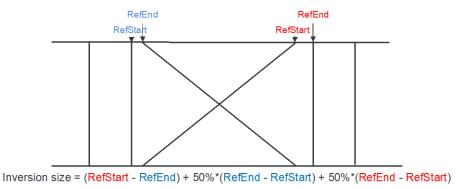
Figure 33. Estimation of inversion size on paired inversion calls.
